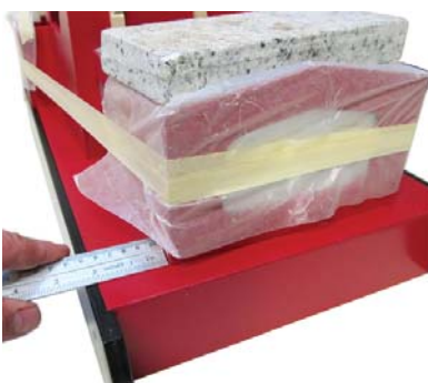
Check again that the Hood Support Set is centered
