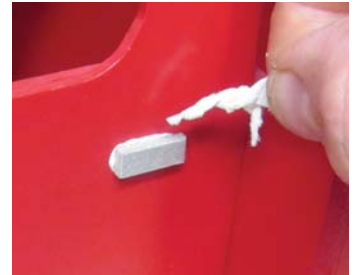
A 5 : Clean up excess glue
